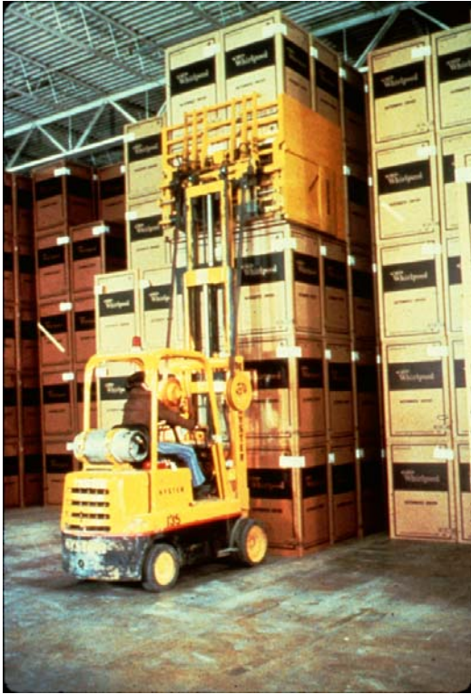
Figure 16.37. Block Stacking Storage Example
